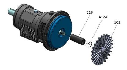
Figure 52: Shaft Sleeve installation
