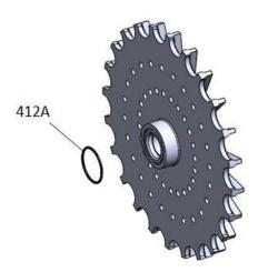
Figure 5: O-ring for models PWA, PWA-LF, PWA-SP
