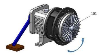
Figure 4: Impeller removal
