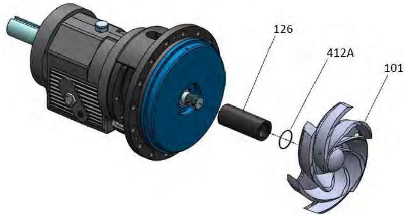
Figure 69: Shaft Sleeve installation
