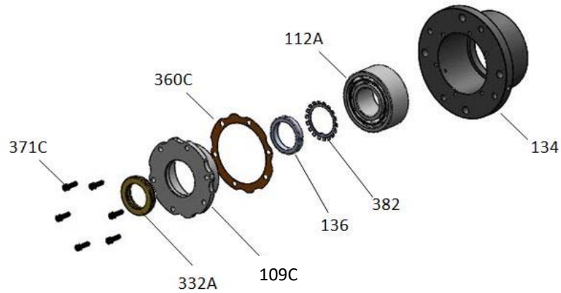
Figure 26: Bearing housing disassembly – Group 4
