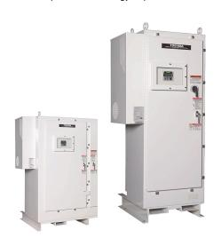
protection. The Plus Pack is a solid-state AC drive that ranges from 66-1500 KVA and features true torque control enabling motors to develop high starting torque and compensating for motor slip. Available in NEMA 3R enclosures, ASD rated for 50 degrees C and 4500 fasl with no derate of output current. The enclosure cooling
