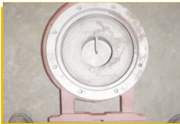
During the inspection process some erosion was found near the suction nozzle. This case will be weld-repaired, stress-relieved and an NDE performed to test the integrity has been restored.
