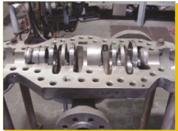
This case has been planed and bored and is in final inspection. Each volute throat area has been inspected and ground to match a template provided by engineering.
