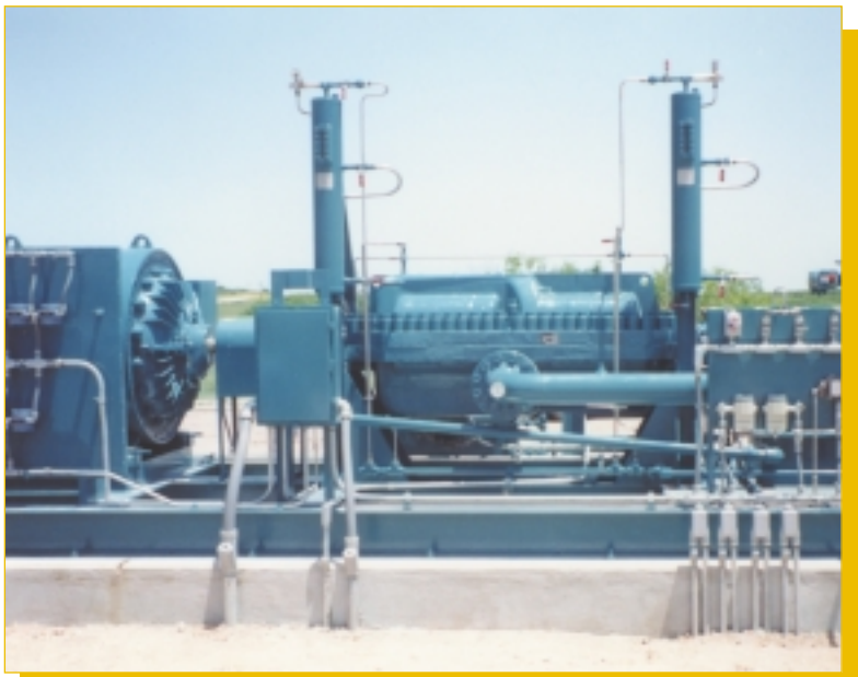
PumpWorks remanufactured Bingham MSD 6X8X11D -10 stage for natural gas liquid, 0.49 spgr. Pipeline application. Unit complete with tandem seals, plan 52, lube oil system and 800 hp motor. Unit shipped in 12 weeks.
