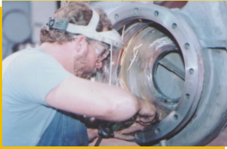
Single stage casing being reworked to match impeller for hydraulic rerate.
