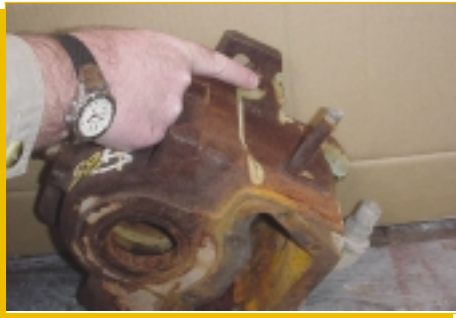
During the preliminary inspection of this bearing housing a piece of the support was found to be broken off requiring the housing to be replaced.
