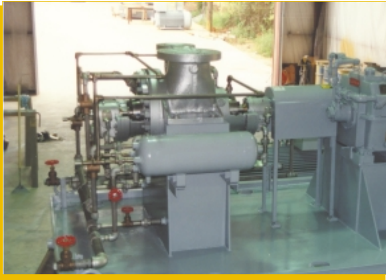
Crude service pump for a Romanian refinery. PumpWorks remanufactured Pacific API 610 4x15 pump with Lufkin speed increaser, Plan K cooling water piping, 6000V/3/50 European specification motor drive. Unit remanufactured, tested and shipped in 12 weeks.
