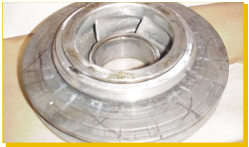
The impeller pictured here has cracks in the shroud that are irreparable. As a result this impeller will not be used in the remanufacturing process.
