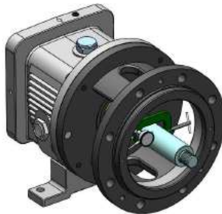
Figure 64: Indicator installation – Frame adapter runout
