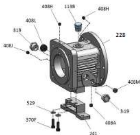
Figure 42: Assemble the bearing frame and foot
